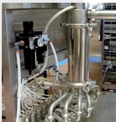
Dosymix Multi outlet feeding downstream dosing heads
