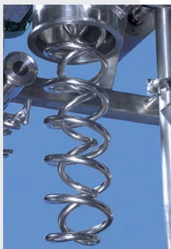
Low shear screw profile preserves product texture
